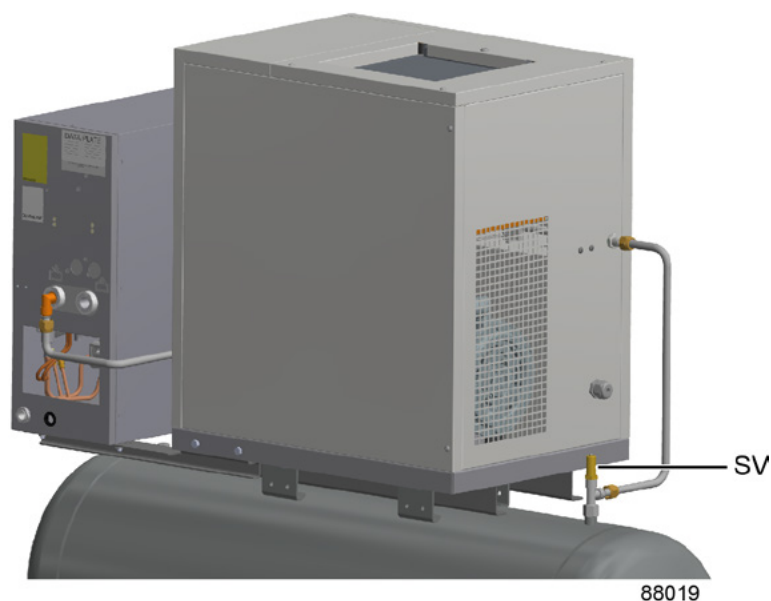
Figure 4: Safety valve on the compressor and on the vessel
